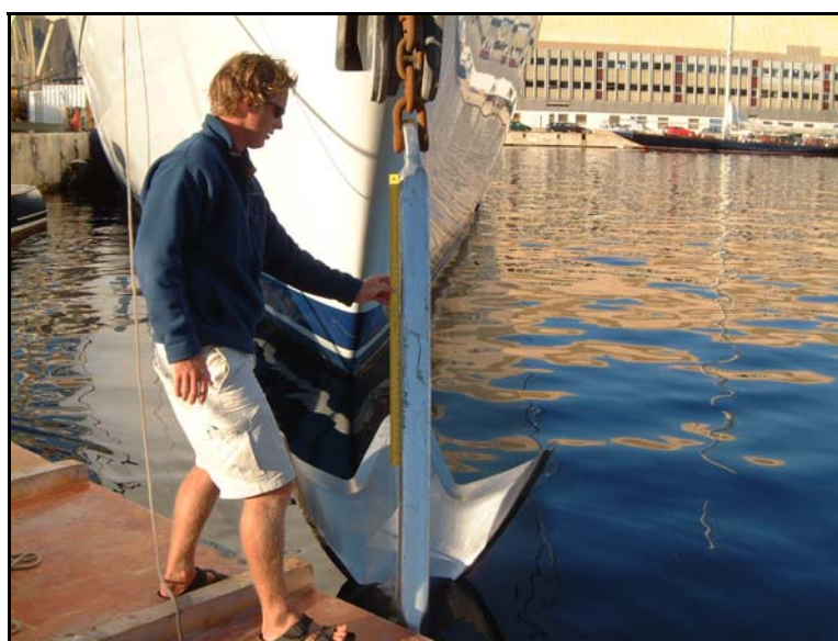
Figure No. 4 Anchor shank deflection against a straight edge
